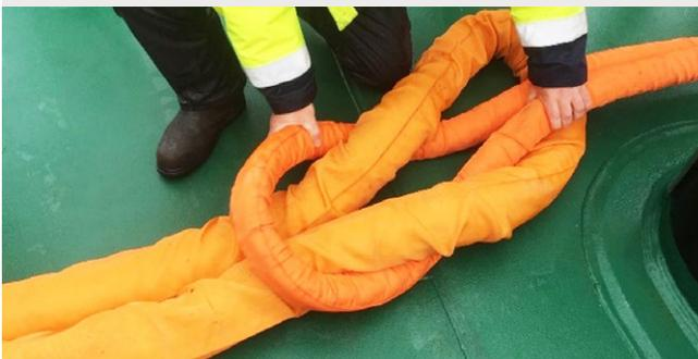
A **cow hitch** can be considered if one length is short and easy to handle like a pennant. The cow hitch in practice can be difficult to get the knot out. A soft round sling tied on the top of each eye can help to separate them.
