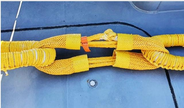
A **soft shackle** can be used that has a matched MBL to the two joined ropes, this is a light option but needs to be fitted on protected eyes to minimise chance of cutting into the joined ropes due to smaller diameter.
