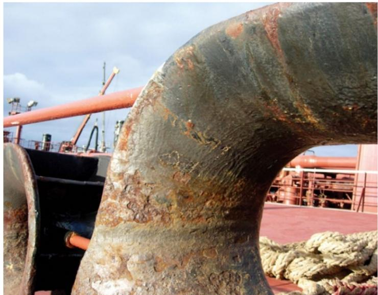
Tow lines should not be exposed to sharp edges and surfaces such as steel-wire gouge marks or metal burrs (on equipment such as winch drums, sheaves, shackles, thimbles, wire slings etc). When replacing winch lines, care must be taken to ensure the rope is not coming into contact with hardware that has been scored or chewed by previously used wire lines.
