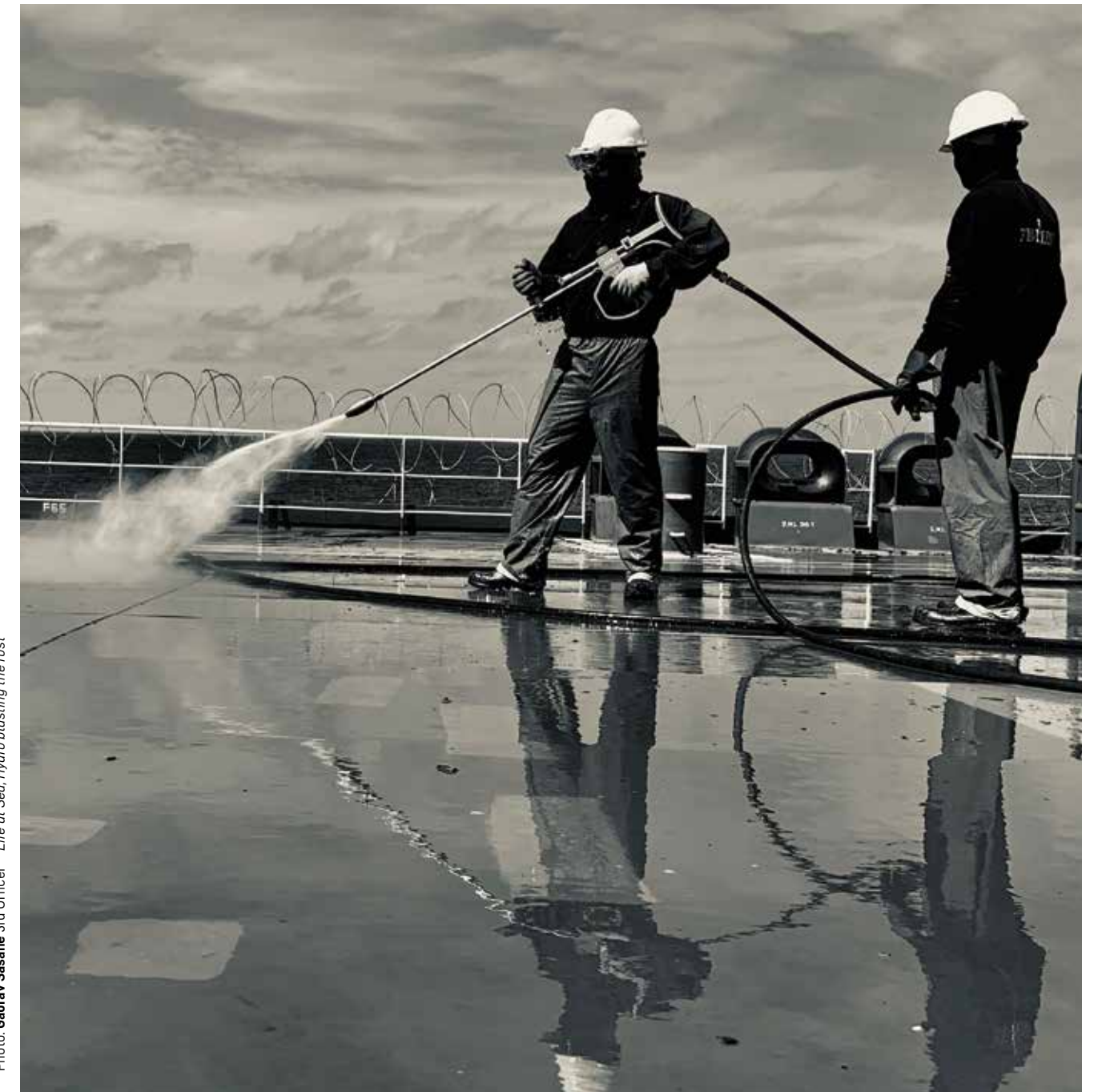
Photo: Gaurav Sasane 3rd Officer - Life at Sea, Hydro blasting the rust
