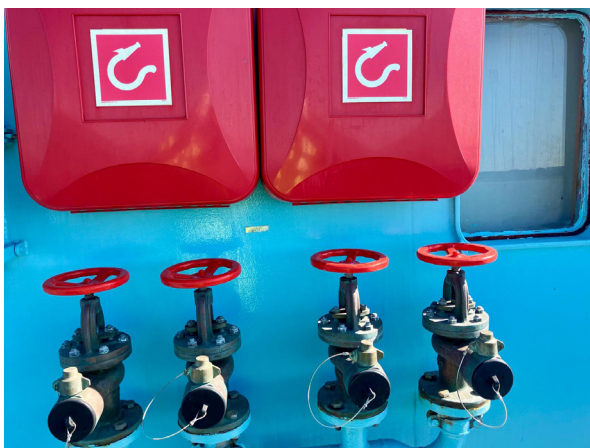
8 x 2.5" hose manifolds, 4 port and 4 starboard on the main deck
