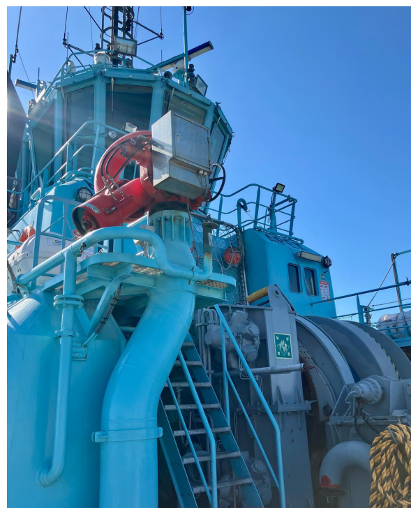
2 x 2000m 3 /hr combined foam & water monitors, one port, one starboard aft
