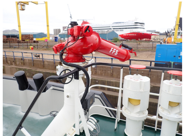
Tug with monitors at wheelhouse level
